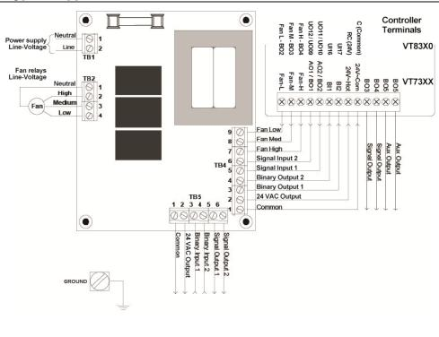
THE CONTACT CONVERTER MUST BE CONNECTED TO EARTH WITH THE AID OF THE GROUND LUG LOCATED ON THE METAL BASE
