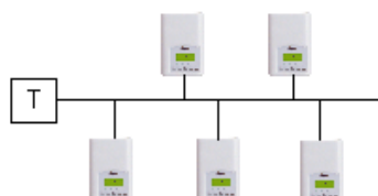
Figure 3.1 Singly Terminated Bus Topology
